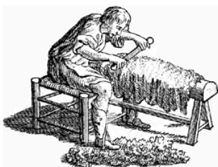
Krünitz Vol. 27 (1783), Fig. 1506, Article ›Hut‹ (Hat): Enthaaren eines Biberfells.
